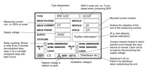
**Note:** The relay is provided with a 200 ms power-up relay, ensuring correct function of the relay on connection of the auxiliary voltage. Normally energized contacts ("NE") are not activated (contact does not open/close) until 200 ms after connection of the auxiliary voltage.
